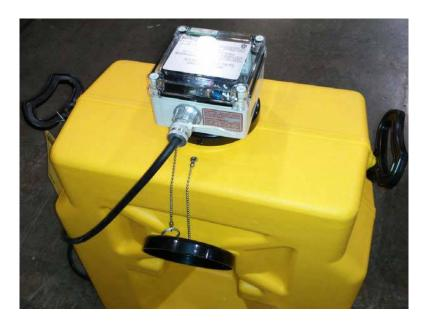
3. Gently rotate the heater approximately  $10^{\circ}$  clockwise and counterclockwise and then back to the center, making sure the heater element does not touch the inside of the tank walls. Adjust rotation if needed to insure element is centered between tank walls.
