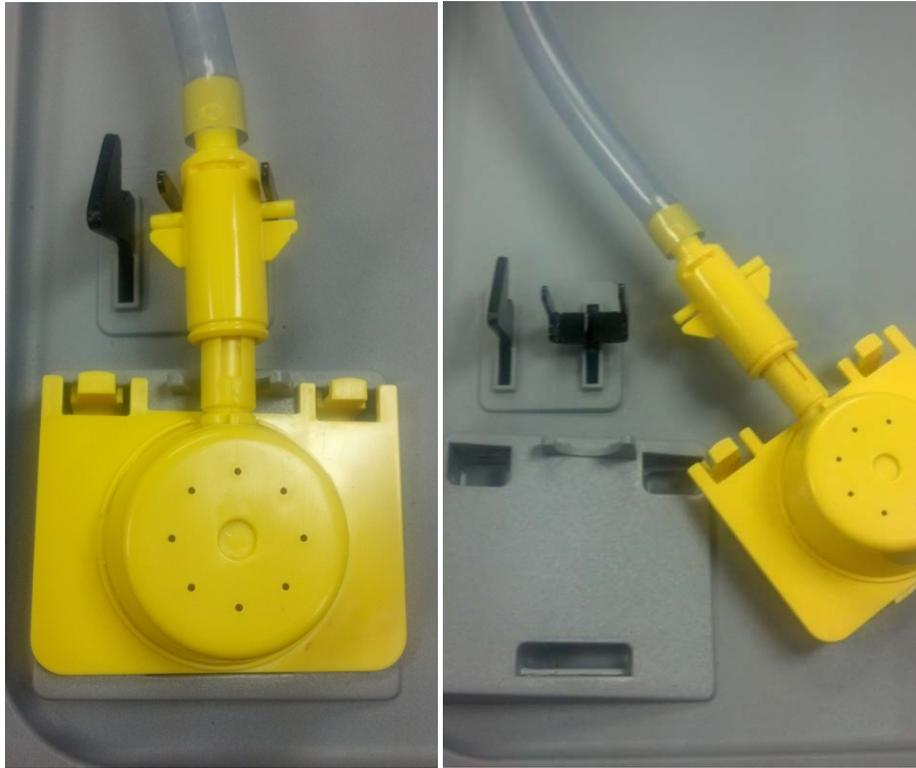
Figure 4: Nozzle Assembly Removed
