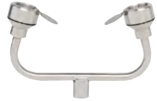
Model 01052263 Eyewash Assembly, SS Heads & Wye, w/Hinged Covers, 1/2" / 1.3 cm Inlet, 2.5 gpm / 9.5 lpm
